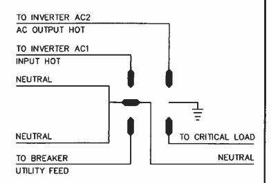
IN POWER OUTAGE, AC1 IS DISCONNECTED BY ELECTRONIC BREAKER AND UTILITY IS ISOLATED FROM GENERATION. DISPLAY ON METER IS NOW OFF AND NO GENERATION IS METERED.
