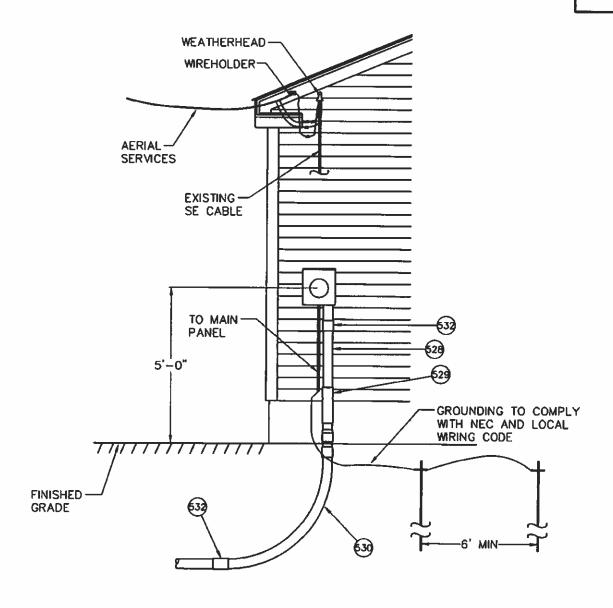
1. REFER TO CONDUIT USAGE CHART FOR CONDUIT REQUIREMENTS.
