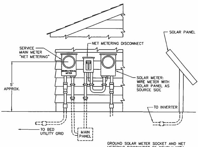
GROUND SOLAR METER SOCKET AND NET METERING DISCONNECT TO COMPLY WITH NEC AND LOCAL WRING CODE.
